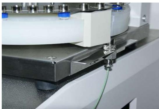
**Fig. 3 Injection port under the carousel**
