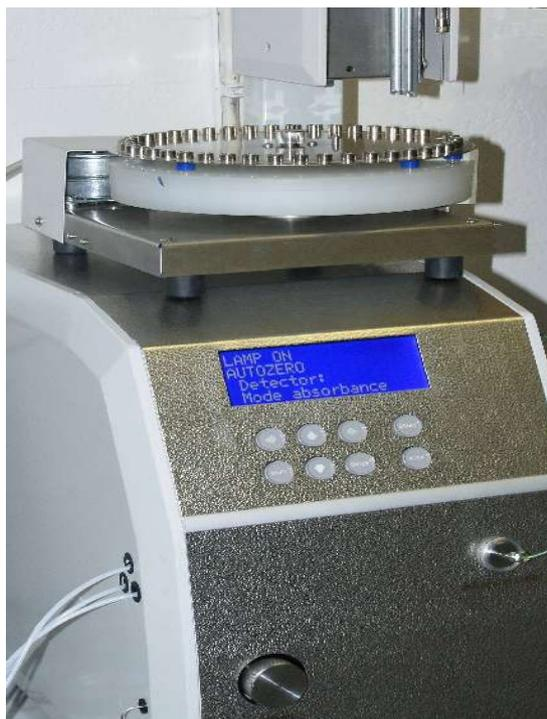
**Fig. 2. Carousel part on the chromatograph**
