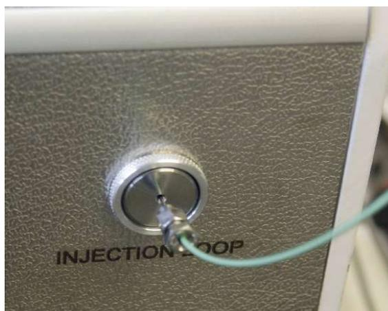
**Fig. 5 Chromatograph injection port**
