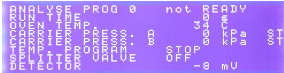
First line of the display indicates program number (from a memory) and at the moment status (not READY, READY, RUN, STOP, COOLING).
