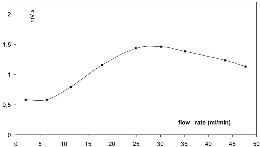
**Fig. 12 :Dependence of peak area on carrier gas flow rate.**
