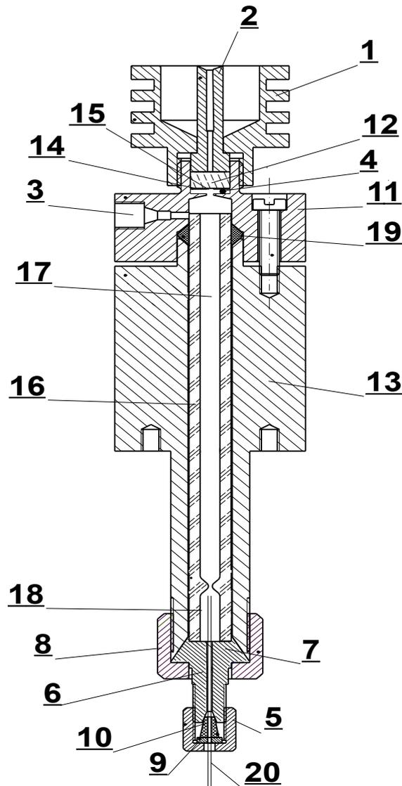
**Fig. 9: Cross – section of the injector block with attached capillary column**
