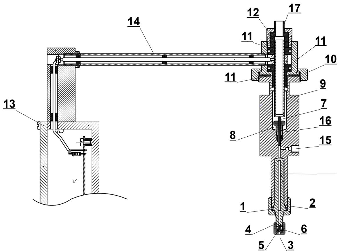
**Fig. 10 : Cross section of the FID. Attachement of a capillary column**
