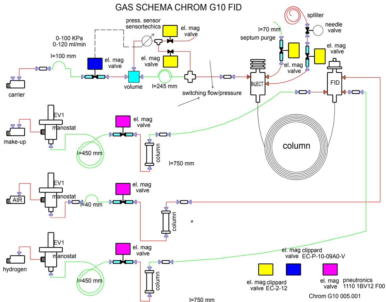
**Fig. 5 : The gas distribution in FID channel**
