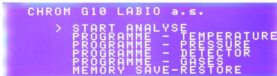
is displayed and the gas chromatograph then goes directly to analyses or over to the mode where individual operating conditions can be entered. Left side arrow indicates which part of the menu will be selected using ENTER button. Using START ANALYSE choice, the display indicates the instrument status:
