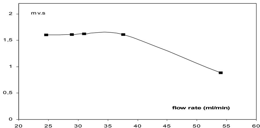
**Fig. 13 : Detector sensitivity as a function of hydrogen flow rate.**
