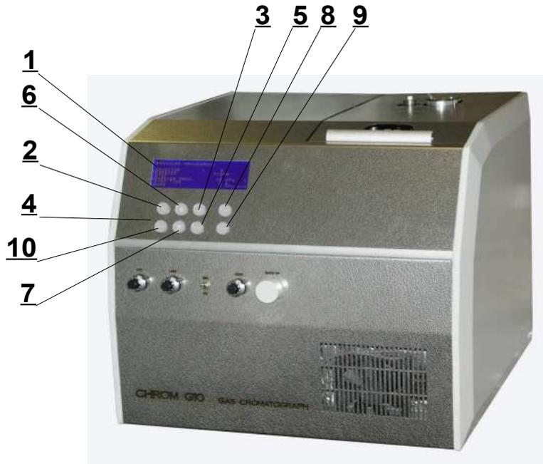
**Fig. 1 : The front panel of gas chromatograph**
