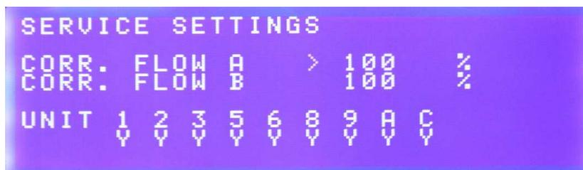
Service settings allows to calibrate carrier gas flow rates depending on the type of gas used. This process is reserved for servicemen only. Last two lines are used to check a function of electronic boards.
