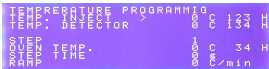
On the second line injector and on third one detector temperature can be set in each case confirmed by ENTER. Heading plates are common for A and B channels and only one value is set for both. Number of a step (1 - 5) is then selected on next row and giving step oven temperature, step time and a ramp parameters are defined. For example if you like to program a standard analysis with one temperature increase, following data are entered
