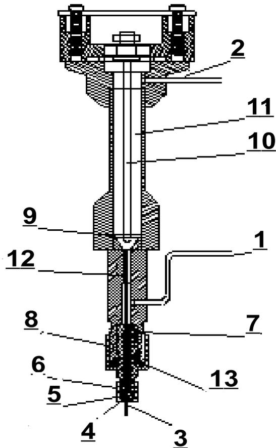
**Fig. 11: ECD detector cross section**
